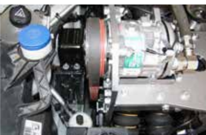
From left: air compressor in the engine compartment; built custom-made air compressor with motor mounting; air compressor
