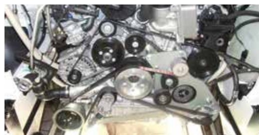
From left: air compressor in the engine compartment; built custom-made air compressor with motor mounting; air compressor
