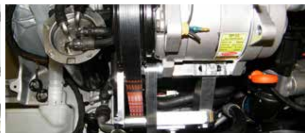
From left: air compressor in the engine compartment; built custom-made air compressor with motor mounting; air compressor
